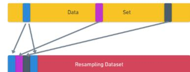
Figure 7. Bootstrap Resampling Method.
